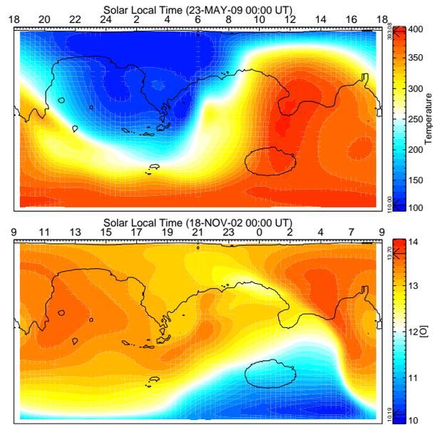
Figure 9: M-GITM results for (top) exospheric temperatures during Mariner conditions and (bottom) O density during Viking Conditions.
