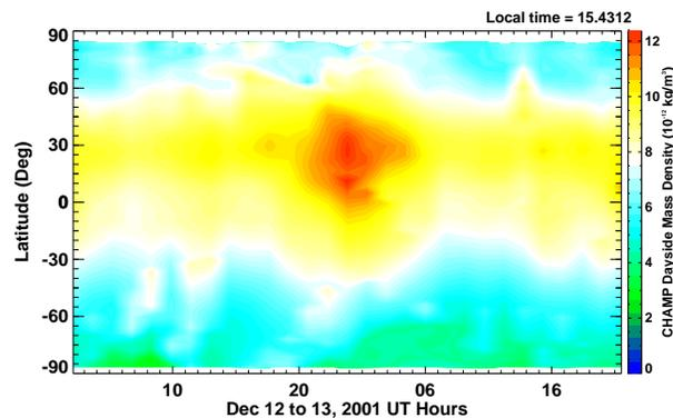
Figure 8: The terrestrial thermospheric density at 400 km as measured by the CHAMP satellite on December 12 - 13, 2001 during several repetitive solar flare events.
