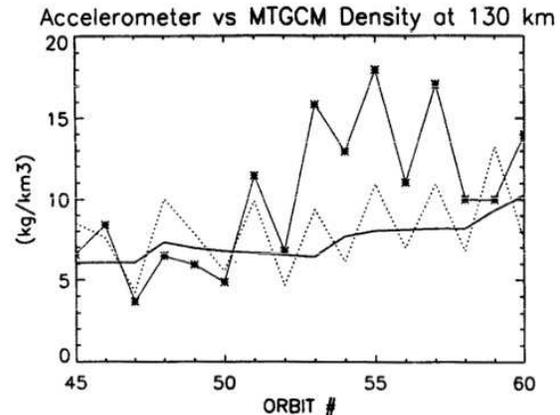
Figure 3: MGS accelerometer densities near periapsis (asterisks) as well as coupled MGCM-MTGCM results using a spatially and temporally dependent dust optical depth including longitude variations (dotted line) and not including longitude variations (solid line) [Bougher *et al.*, 1999].
