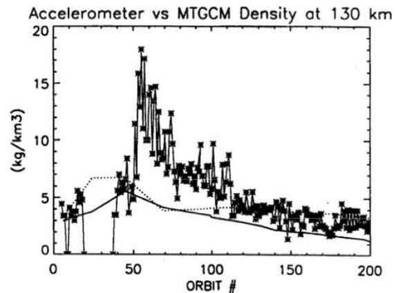
Figure 2: MGS accelerometer densities near periapsis (asterisks) as well as coupled MGCM-MTGCM results using  $\tau = 0.3$  (solid line) and  $\tau = 1.0$  (dotted line) [Bougher *et al.*, 1999].
